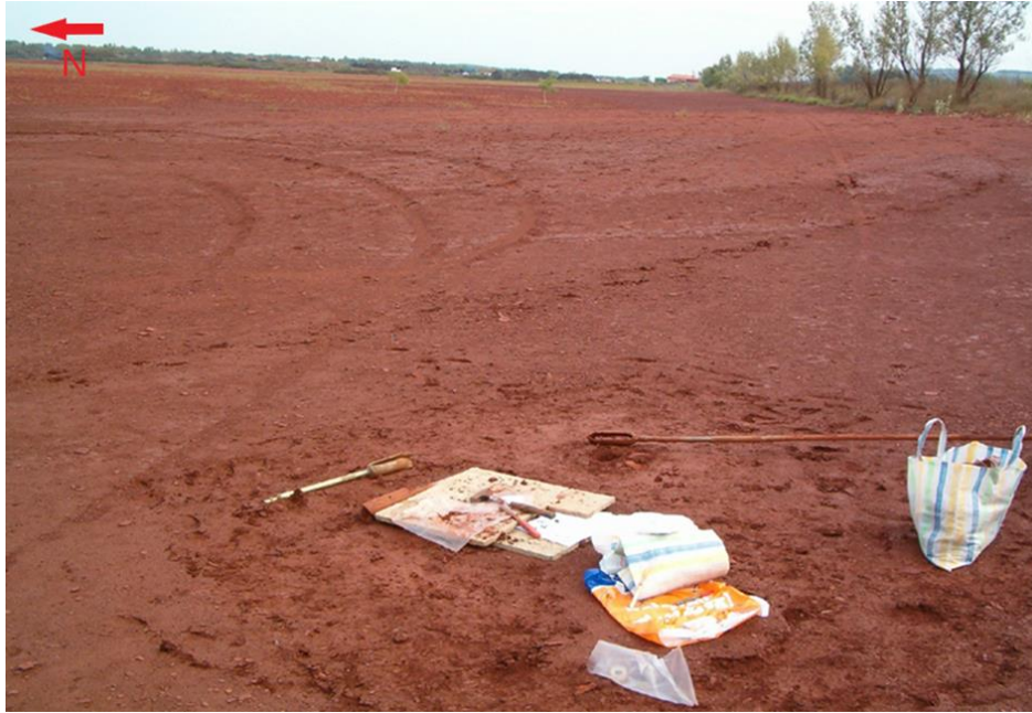
Figure 10E. Sampling process in Almásfüzitő red mud cassette at Ny1 drilling point. The sampling was carried out by soil hand drill.
