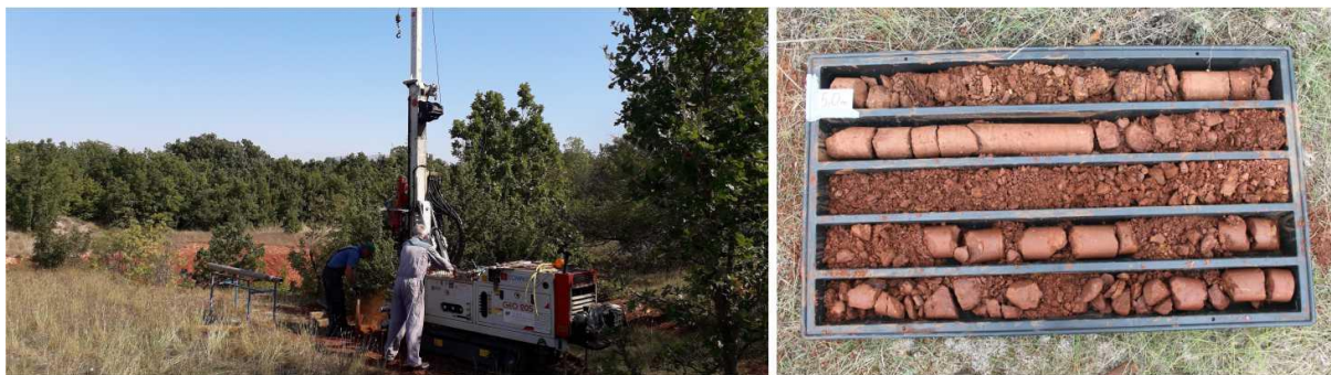
Figure 3. Drilling at Mamutovac 1A deposit (left) and a section of the collected drilling core (right).
