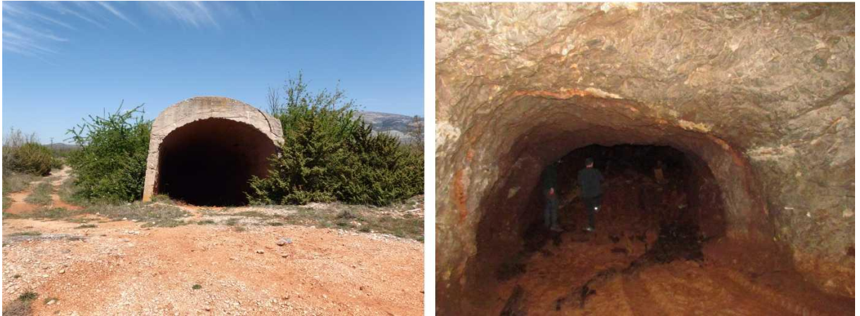
Figure 5D. Entrance (left) to the underground bauxite mine (abandoned) in Jukići-Đidare and contact of the hanging wall rock (limestone) with bauxite body within the mine (right).
